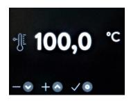
Use keys 1 and 2 to set the required temperature value, confirm with key 3 and return to the main menu. The set point is now displayed beneath the temperature symbol in the main menu.
