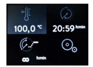
Keys ① and ② permit to move in the menu. The current function is marked in gray and can be opened with key ③. If the saved set points below the function symbols are in conformity with your process requirements, the Water Bath can be started by pressing key ④ (keep pressed for 3 seconds) and switched off again by pressing key ④ (shortly).
