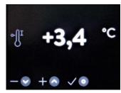
The switch-on point for the over-temperature alarm can be set between  $0.0~\rm K$  and  $+10~\rm K$  above the set point temperature. The switch-on point for the under-temperature alarm can be set between  $0.0~\rm K$  and  $-10~\rm K$  below the set point temperature. Only if process-related and absolutely unavoidable, should the value for the under-temperature alarm be set lower than  $-4.0~\rm K$  and the over-temperature alarm to values lower than  $+2.0~\rm K$ .
