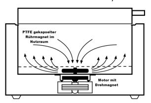
The circulation system ensures an optimized temperature distribution throughout the whole Water Bath. It is operated by an electric motor with stirring magnet, flanged to the Water Bath basin, that transmits its torque to a PTFE-coated stirrer. The stirrer draws the water to the middle of the basin and then moves it back to all sides. The electric motor of the water circulation is activated via the main switch.
