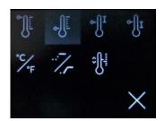
Use keys 1 and 2 to move in the menu. The current function is marked in gray, key 3 opens the input window to define the required pre-set value.
