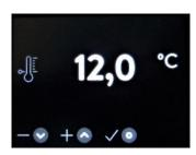
The maximum set point can be defined between  $10.1\,^{\circ}\text{C}$  and  $100\,^{\circ}\text{C}$ , the minimum set point between  $10.0\,^{\circ}\text{C}$  and  $99.9\,^{\circ}\text{C}$ . The values of both functions are interlocked. The maximum limitation of the set temperature cannot be set lower than the minimum limitation and vice versa. Therefore, the temperature can be set and limited between  $10\,^{\circ}\text{C}$  and  $100\,^{\circ}\text{C}$ .
