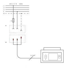
Models H 4, H 8, H 16, H 22, H 24, H 41, H 8 A, H 16 A for 230 V with power supply  $220 \, \text{V} / 3 / \text{N} / \text{PE} / 50/60 \, \text{Hz}$ , connected through 3-pole shock-proof (Schuko) plug system.
