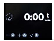
Set the required time value with keys  $\bigcirc$  and  $\bigcirc$ , then confirm with key  $\bigcirc$  and return to the main menu. The set delay will be displayed beneath the symbol of the switch-on delay in the main menu.
