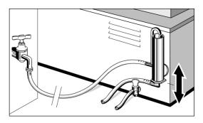
Secure all hose connections with hose clips.
